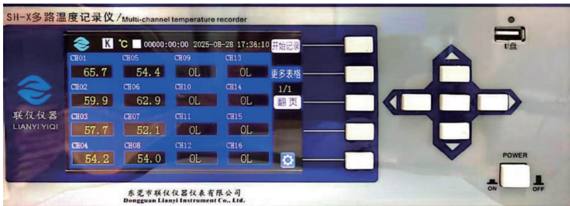
Fig. 2: Multi-channel Temperature recorder
