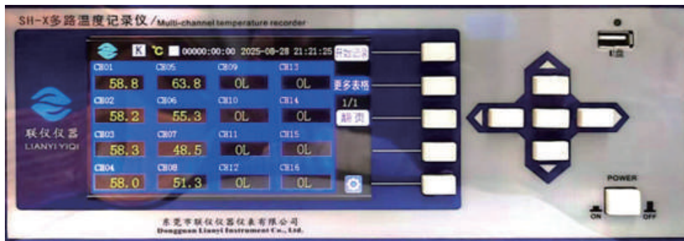
Fig. 2:Multi-channel Temperature recorder
