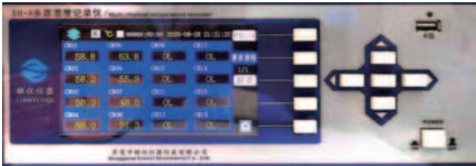
Fig. 2:Multi-channel Temperature Recorder
