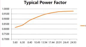
Note: Test data under 700mA gear
