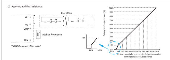
Note: 1. Min. duty cycle of output current is about 6% and the output current is not defined when 0% Iout<6%. 2. The duty cycle of output current could drop down to 0% when dimming input is about 0% or 0% or 0% or 0% or 0% duty cycle.
