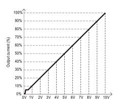
Dimming input: Additive voltage
