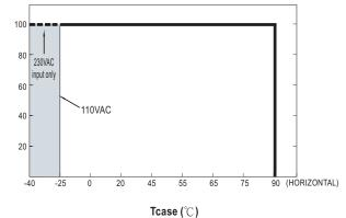
If ELG-240 operates in Constant Current mode with the rated current, the maximum workable Ta is 60°C.
