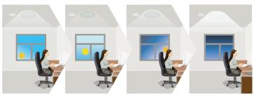
The light turns on at full or dims to maintain the lux level. The light output regulates accroding to the level of natural light available.
