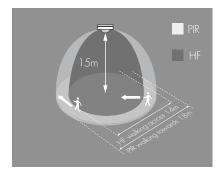
PIR detection:  $H \times D:15 \times 18m$  (max. ) HF detection:  $H \times D:15 \times 14 m$  (max. )
