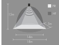
PIR detection:  $L \times W \times H$ :  $18 \times 5 \times 15$ m (max.) HF detection:  $H \times D:15 \times 14 m$  (max. )
