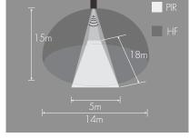
PIR detection:  $L \times W \times H:5 \times 18 \times 15 m$  (max.) HF detection:  $H \times D:15 \times 14 m$  (max. )
