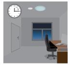
The light dims down and eventually turns off when the ambient natural light is sufficient.
