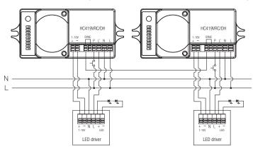
\*If required - (no earth connection neccessary on HC419VRC/DH)
