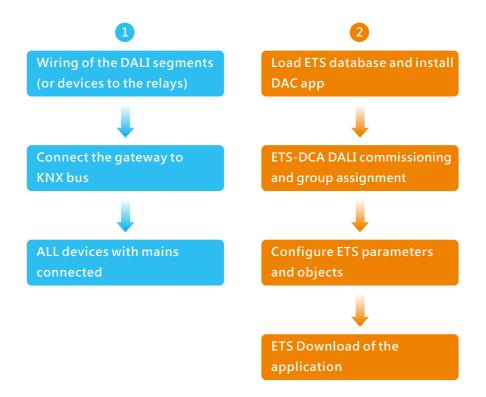
After the wiring of the DALI segments according to instructions in the following sections, software start-up can begin. To do this, the product database is loaded and the corresponding ETS App is installed in the ETS, see 3.5 ETS App (DCA).
