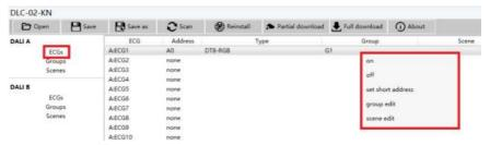
Command 1: ECG-on Turn on the ECG.
