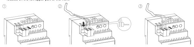
c. Connect the mains voltage, the connection to the AC is made with the terminal (L, N,  $\frac{\perp}{=}$ ) located on the bottom.
