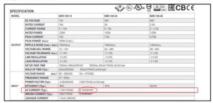
Check AC input current spec of SDR-120-24 and do calculation with the rated current of ICL-16
