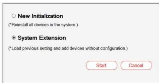
※"Initial Installation": All devices on the DALI bus are re-addressed, but the previous parameters of devices remain unchanged.
